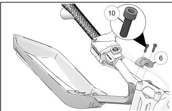
6. Carefully rotate the handguard assembly upward and into position.
